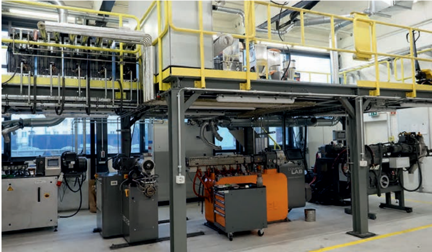
Up to five systems can run simultaneously in the pilot plant. The material feed is provided by means of feeds from the upper level. © Hanser/Schröder
