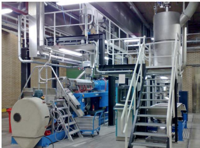
Fig. 3. At the heart of the PVC line is a high-performance Kneader with cascade pelletizer
