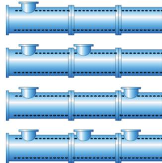
A third barrel module extends the processing length to 11 L/D. Barrel modules with and without feed ports can be combined at will. Thus, raw material components can be fed downstream into the Buss Kneader; a feature increasing the versatility and flexibility in processing.
