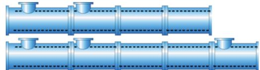
Four barrel modules result in a total processing length of 15 L/D. Again the barrel modules can be equipped with feed ports for feeding or for devolatilization.
