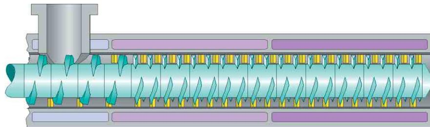
The barrel modules are jacketed for the circulation of a fluid heat transfer medium. As a result and similar to the kneading screw the entire surface of the barrel contacted by the stock is precisely temperature controlled. According to the process requirements the barrel modules can individually set to different temperatures.
