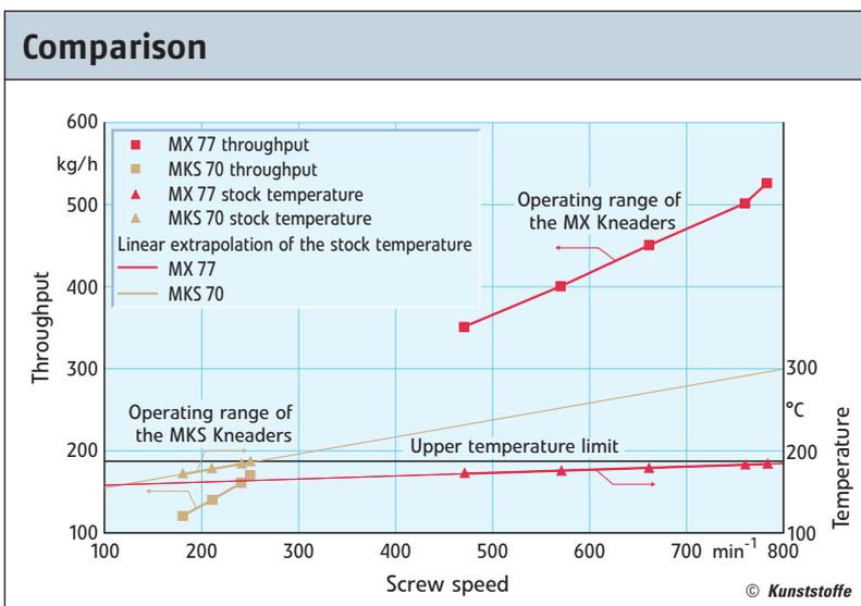
**Fig. 3. The plot of stock temperature and throughput versus screw speed shows clearly the improvements in the MX Kneader over the previous MKS Kneader**
