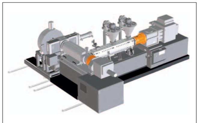
**Fig. 1.** Major parts of the high-performance MX Kneader Series: motor-gearbox unit, processing section with feed locations, directly flange-mounted single-flight discharge screw with melt filtration and pelletizing
