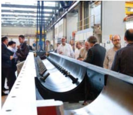
Fig 3. The removable kneader upper housing is easily accessible on the service station right
