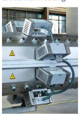
The process area is electrically heated. This concept prevents additional installation cost compared to liquid heating (HTM).
