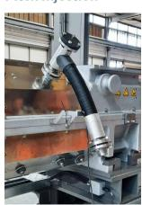
In the transition section, liquid pitch is directly injected into the feedstock via drilled kneading bolts.
