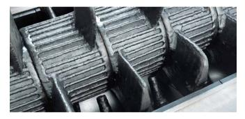
In the kneading and mixing section, the focus is on optimum mixing. Innumerable flow separations and reorientations with uniform shear rates ensure maximum homogeneity. This leads to optimised performance of the final anode product.
