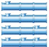
A third barrel module extends the processing length to 11 L/D. Barrel modules with and without feed ports can be combined at will. Thus, raw material components can be fed downstream into the Buss Kneader; a feature increasing the versatility and flexibility in processing.
