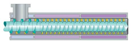
The barrel modules are jacketed for the circulation of a fluid heat transfer medium. As a result and similar to the kneading screw the entire surface of the barrel contacted by the stock is precisely temperature controlled. According to the process requirements the barrel modules can individually set to different temperatures.
